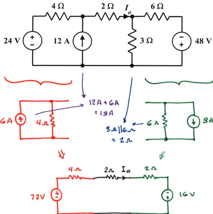
$$I_o = \frac{72V + 16V}{4\Omega + 2\Omega + 2\Omega} = 11A$$
